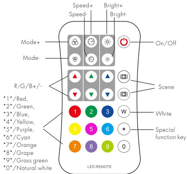
**Mode+/-:** Short press switch dynamic mode built in controller, long press 2s Mode+ run mode cycle, long press 2s Mode- run the first mode. Default 32 dynamic modes, long press the Mode+ key for 2s will automatically get the current number of dynamic modes of the controller.
