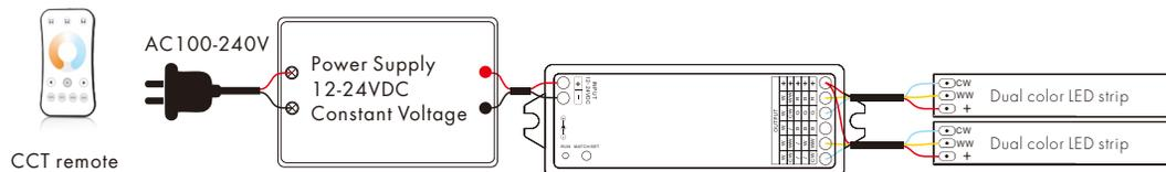
Press and hold match/set key for 10s, until the RUN LED indicator turn yellow, then release, the controller will become CCT type, then do smart config by tuya APP, or short press match key to match with CCT RF remote.
