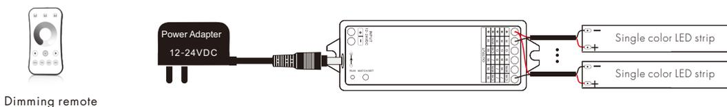
Press and hold match/set key for 8s, until the RUN LED indicator turn white, then release, the controller will become DIM type, then do smart config by tuya APP, or short press match key to match with dimming RF remote.
