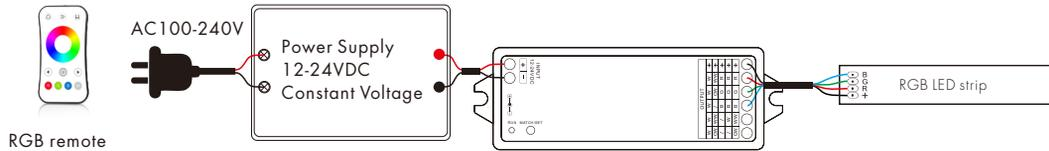
Press and hold match/set key for 12s, until the RUN LED indicator turn red, then release, the controller will become RGB type, then do smart config by tuya APP, or short press match key to match with RGB RF remote.
