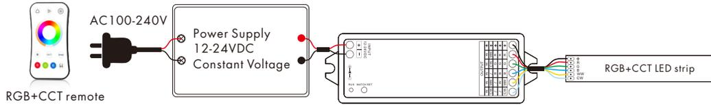
Press and hold match/set key for 16s, until the RUN LED indicator turn blue, then release, the controller will become RGB+CCT type, then do smart config by tuya APP, or short press match key to match with RGB+CCT RF remote.
