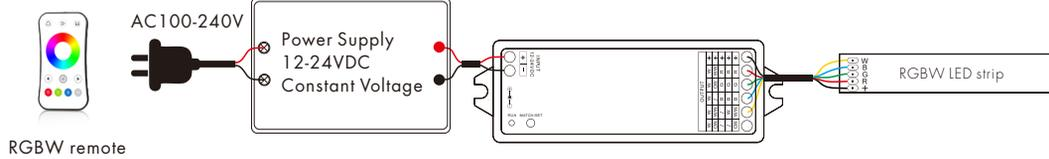
Press and hold match/set key for 14s, until the RUN LED indicator turn green, then release, the controller will become RGBW type, then do smart config by tuya APP, or short press match key to match with RGBW RF remote.
