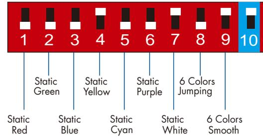
1. For dynamic effects (DIP Switch 8,9 = on) : DIP switch 1-7 is used to get 7 speed levels. (7=on, the fastest level)
