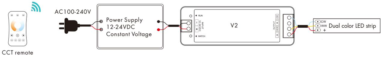
Note: Continuously switch off and on the power supply two times rapidly, It will change 3 levels color temperature (WW, NW and CW) in sequence.
