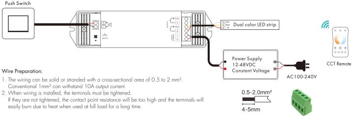
Note: 1. Continuously switch off and on the power supply two times rapidly, It will change 3 levels color temperature (WW, NW and CW) in sequence.
