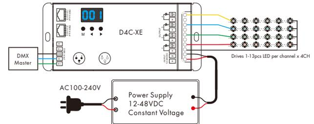
1. The LED quantity at each channel can be different, the decoder could auto check and output a proper voltage to each channel according to its LED quantities.
