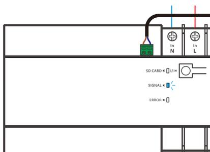
After powering on, the device will enter the Bluetooth Pairing Mode during the first use. The Signal Indicator flashes quickly.
