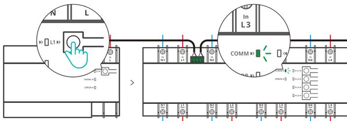
Press the Pairing Button on the main unit once to enable it enter the scan status, then the COMM Indicator of the slave unit “flashes slowly”. The slave unit will appear in the list of main unit interface on the eWeLink App as a sub-device after being added to the main unit.
