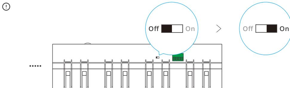
The "RS-485 Termination Resistor Switch" of the slave unit is off by default. To make sure stable communication, the "RS-485 Termination Resistor Switch" of the terminal slave unit shall be turned on.
